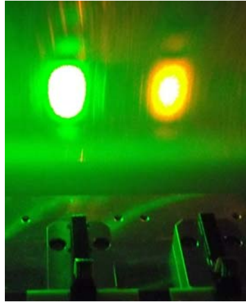
Figure.1 Projected laser light of 561, and 594 nm from the compact laser modules
