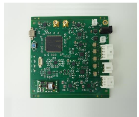
Driver board (option) size (110 x 100 x t16mm)
